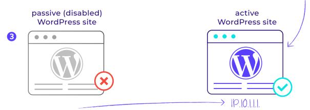
The IP address and the traffic of the malfunctioning stack is transferred over to the newly active one.
